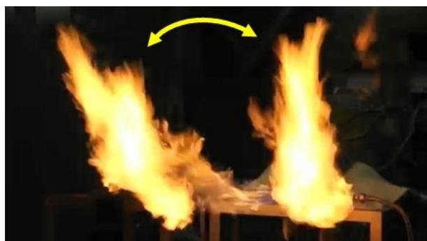
Fig.18 Combustion state of self-induced oscillation burner
