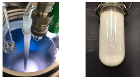
Figure 6 Photos of GaCl<sub>3</sub> solidified in a quartz trap.
