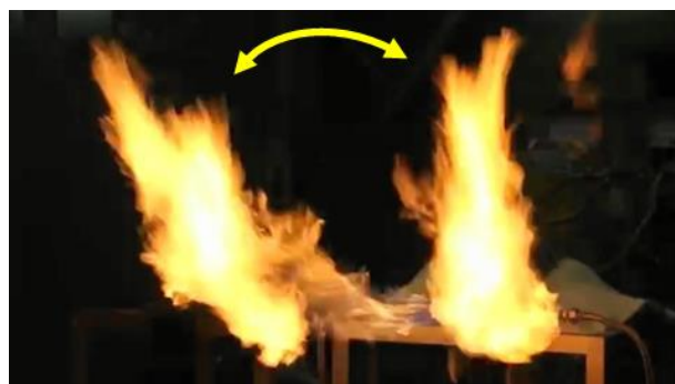
Fig.18 Combustion state of self-induced oscillation burner
