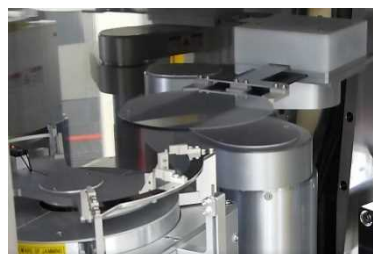
Fig. 3 Robot and aligner for substrate transfer
