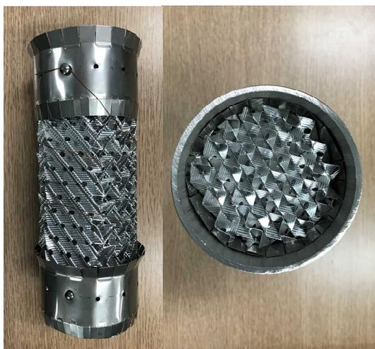
Figure 3 Small-diameter structured packing column
