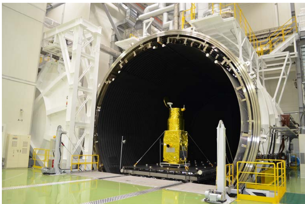
Fig.2 The Large Thermal Vacuum Test Facility Outline (Photo by NEC)
