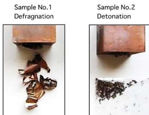
Fig.8 Results of LOX explosion tests(broken fragments)
