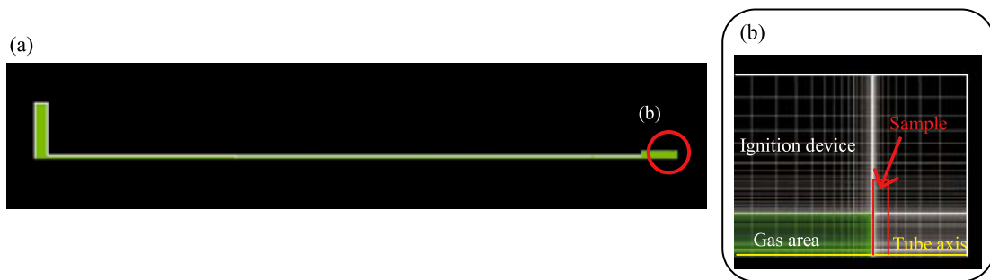
Fig. 2 A schematic diagram of the finite grid. (a) overall view, (b) close-up near the sample
