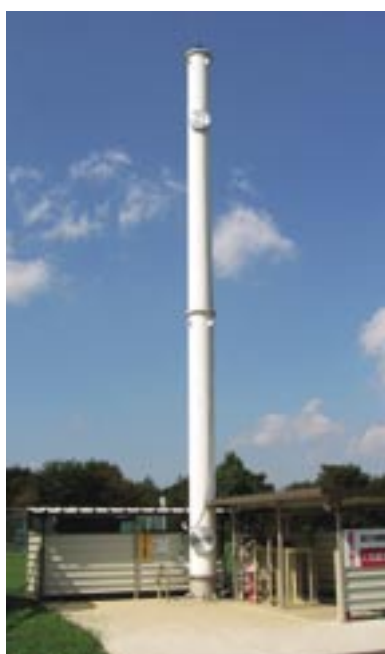
Fig. 5 Pilot-scale oxygen distillation column.
