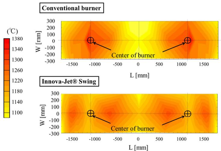
Figure 2: Temperature distribution for base of quasi-tundish vessel
