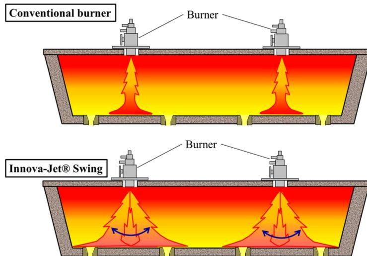
Figure 1: Tundish application for burners
