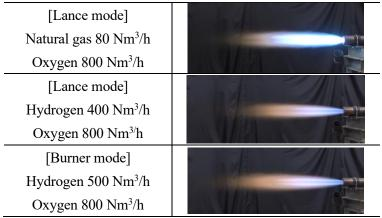
Fig.1 SCOPE-JET<sup>®</sup> combustion flames
