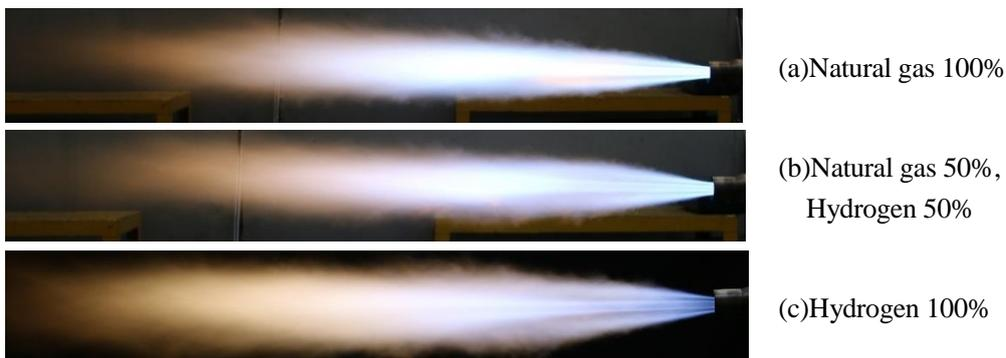
Flame of hydrogen-oxygen burner
