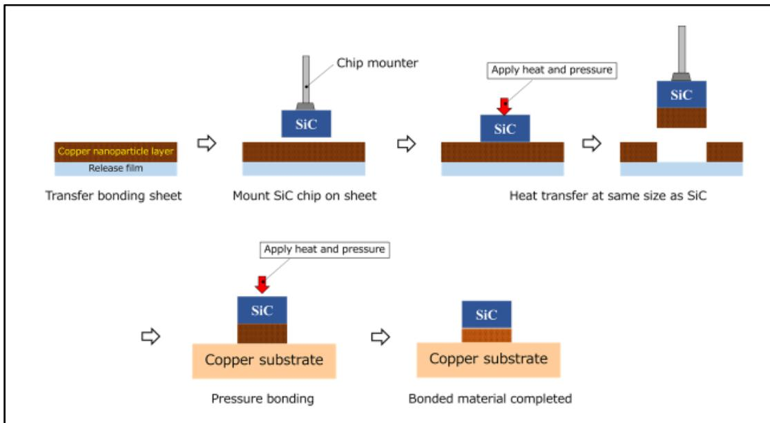
Diagram 1 Overview of transfer and bonding process of transfer bonding sheet
