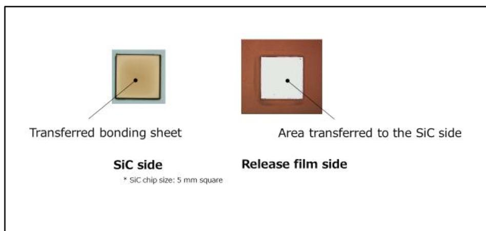
Diagram 2 Exterior view of SiC and release film after transfer of transfer bonding sheet
