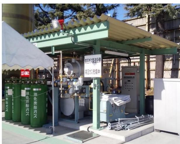
CO<sub>2</sub> liquefaction system
