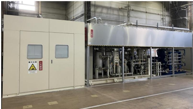
Exterior view of the test equipment used to demonstrate the production of hydrogen from ammonia that meets the fuel quality for FCVs
