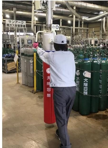
Transporting a high-pressure gas cylinder using the CLifter
