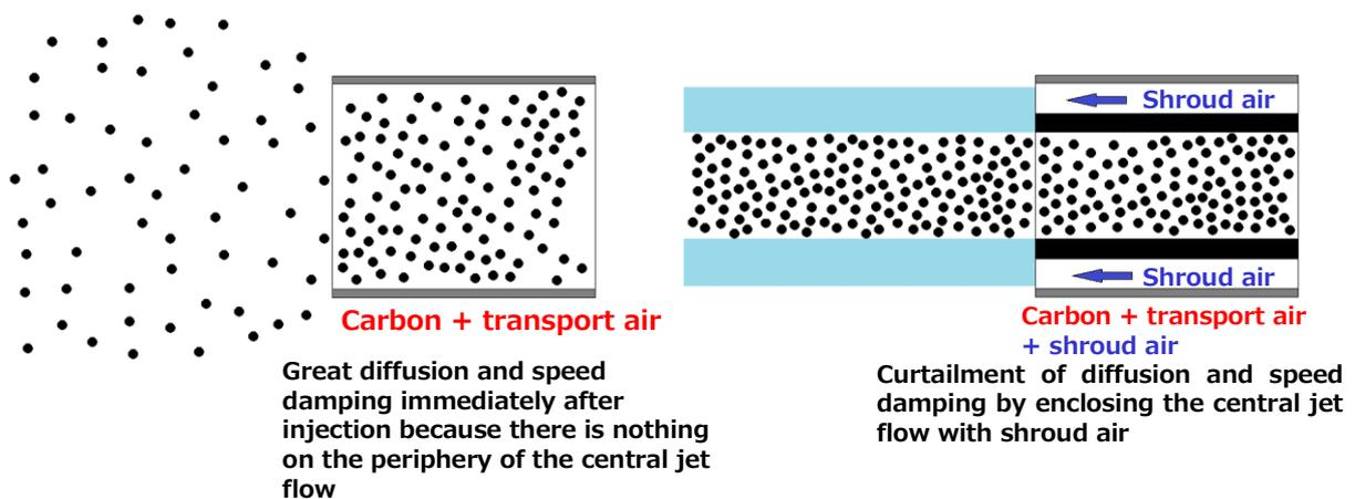
Figure 2 Schematic Diagrams of Jet Flow (left: single-hole lance pipe, right: TSCi)
