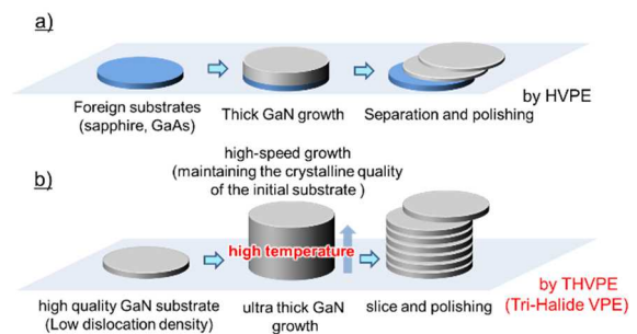
Figure 1 Fabrication of GaN substrate by HVPE and THVPE. The growth scheme in (b) cannot be realized by conventional HVPE.
