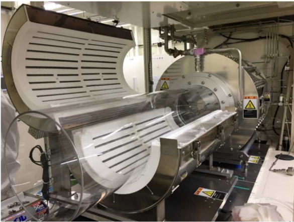
Figure 8 Photograph of THVPE reactor after three years of use (just after washing with water)
