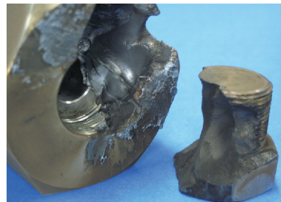
Fig.11 Stop plug appearance damaged by fire
