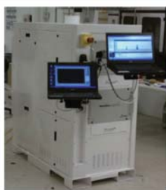
Fig. 1: Photograph of Matheson's AGAS for making DRE measurements from abatement units
