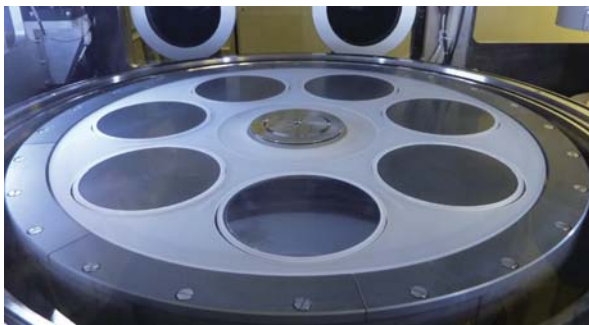
Fig. 2 Susceptor of 6" x 7pcs UR25K MOCVD system
