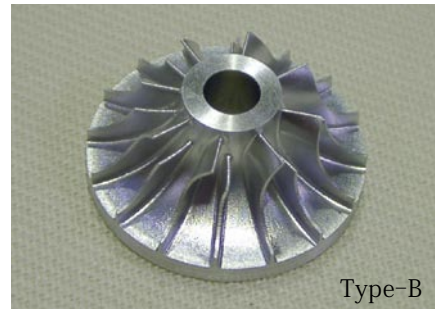
Fig. 3 The photographs of 25 mm turbine impellers, Type-A : 16 full blades, Type-B : 8 full blades and 8 splitter blades.
