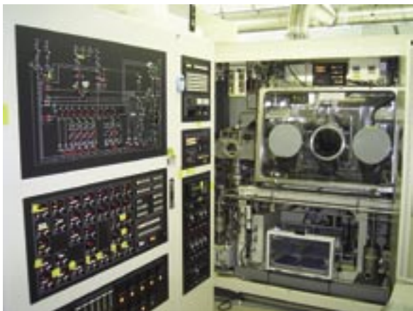
Fig. 1 MOCVD system (SR-4000) in Nagoya Institute of Technology.
