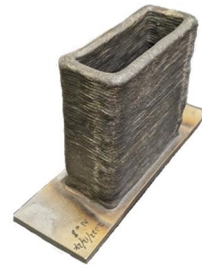
Figure 5 Additive manufacturing sample produced using rotary TIG welding
