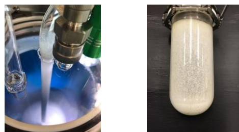
Figure 6 Photos of GaCl 3 solidified in a quartz trap.
