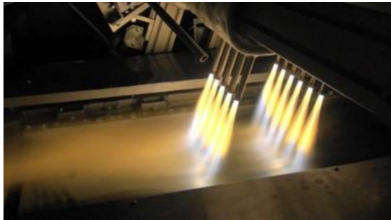
Fig.27 Combustion state of ammonia
