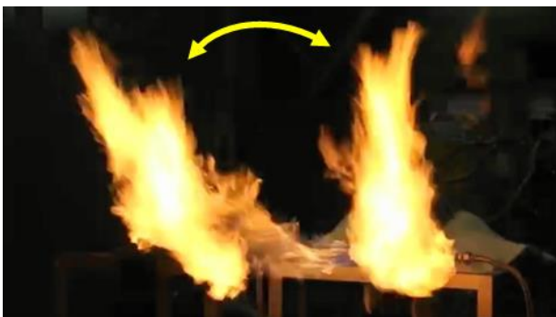
Fig.18 Combustion state of self-induced oscillation burner
