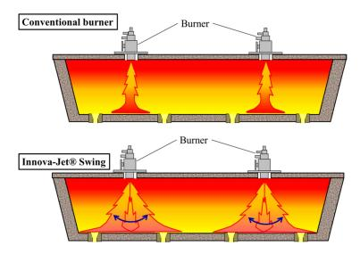
Figure 1: Tundish application for burners
