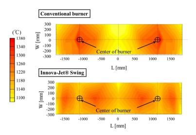
Figure 2: Temperature distribution for base of quasi-tundish vessel
